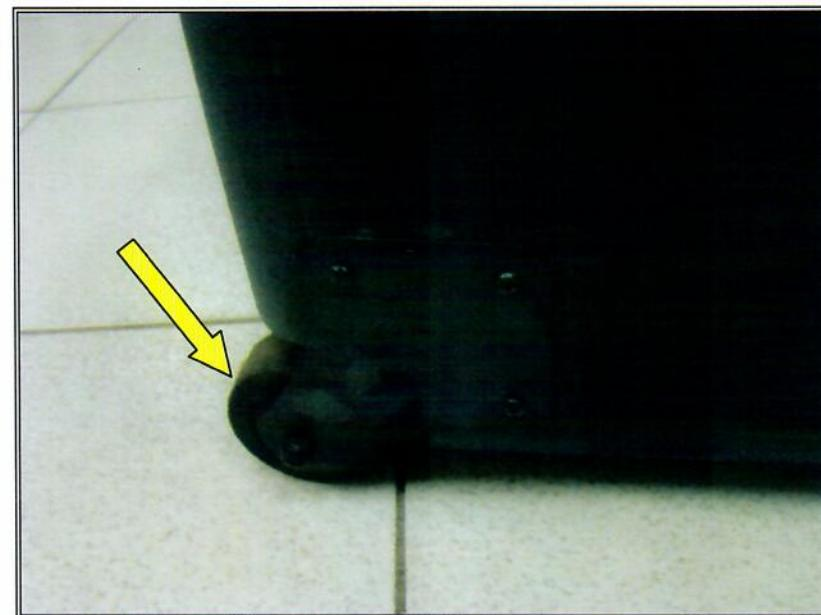
**Figura 30 – Detalhe do rodízio**
